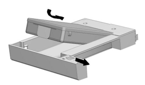
Figure 7-6. Placing a Hard Drive in the Hard Drive Carrier
